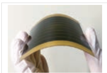
1 Perovskite solar cell flexible minimodule with 20% energy conversion efficiency developed by Segawa lab.
